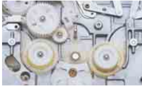
VTR 消音性ギヤ Silent gears for VCRs
