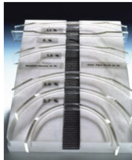
Stencil for strip bending test acc. ISO 4599
